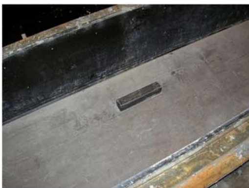
P7. The guiding unit is fasten with two-sided tape or one can use "Uretan Metall", which is an fast drying glue.
