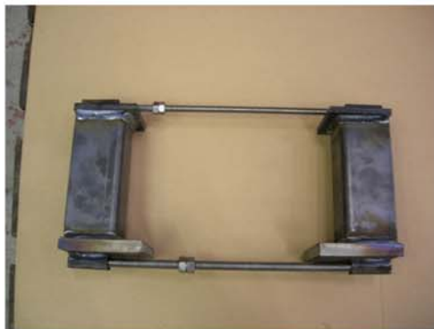
P3. Double column unit, with the threaded bar.
