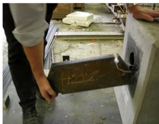
P22. Attach the rope to the knife, and push the knife inside the unit.
