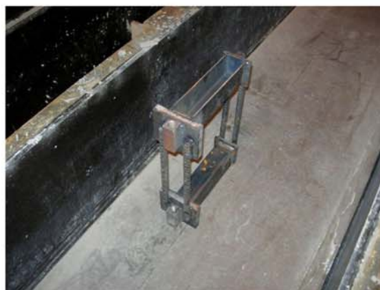
P8. Two- sided column unit placed on the guiding unit.
