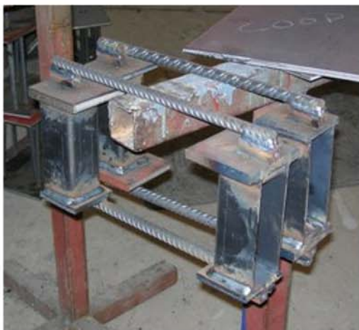
P5. Instead of the threaded bar, one can use welded reinforcement bars.
