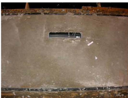
P11. The column unit is embedded in the column.
