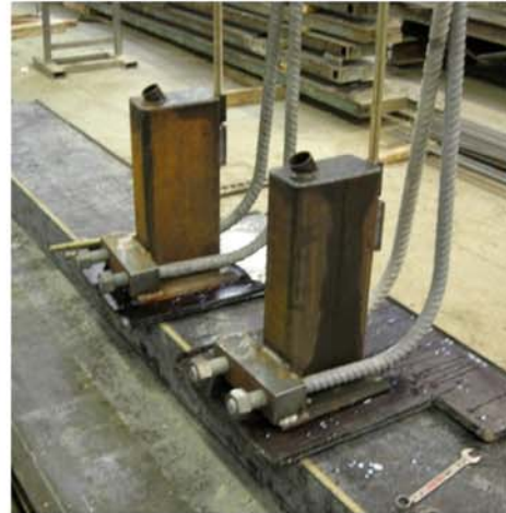
P14. BCC 450 with 2 - Ø32 mm reinforcement bars .
