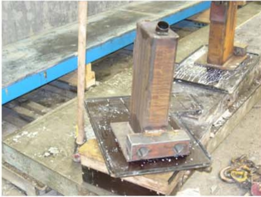
P13. BCC 450 beam unit mounted on the guiding unit.
